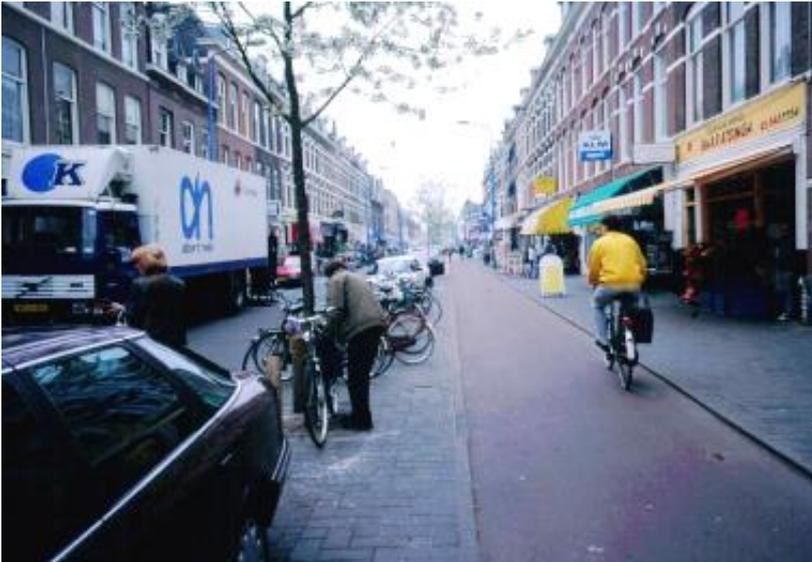
\*An example of how a continuous cycle route, plus accompanying traffic reduction and calming measures, can be created by re-allocating road space by effective segregation. The Hague. This is the model for the Seven Stations Link proposed by Camden Cycling Campaign.\*
