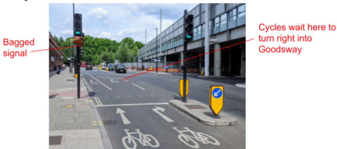
Photo 8. Northbound approach on Midland Road
