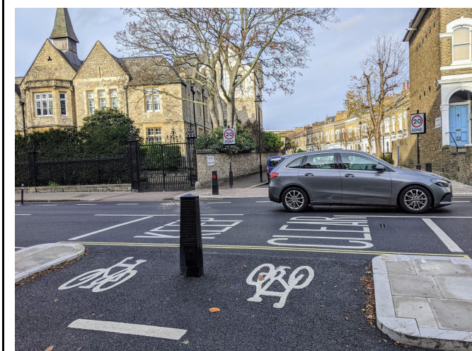
Figure 2. Access to and from to Ryland Road. The KEEP CLEAR allows access in and out of the westbound cycle lane. As eastbound queues sometimes form here, it would be useful to have a KEEP CLEAR in both directions.
