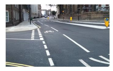
The photo on the left shows the junction of Farrier Street – a good model in that there are clear markings of the cycle track and a logo in front of the exit lane from the side road.
