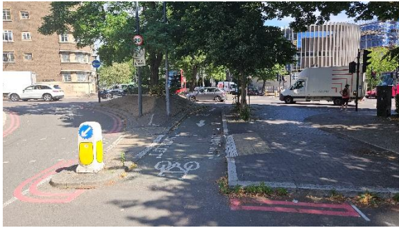
Fig 13.1: St John's Wood Pk modal bypass
